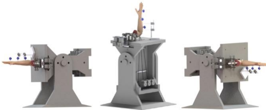
Figure 1.20. Active motion wrist simulator by Iglesias et al. This active motion simulator utilized closed-loop optical control and tests in several gravity-loaded positions. (Reprinted with permission from: Iglesias et al. Thesis Dissertation 2015: Development of an in-vitro passive and active motion simulator for the investigation of wrist function and kinematics).
